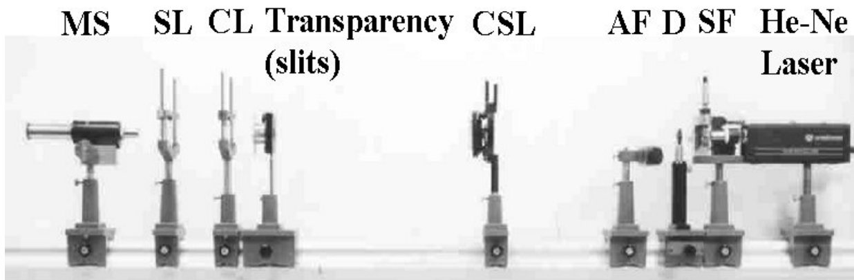
FIGURE 3. A coherent astigmatic optical processor (Experimental setup). A slit is illuminated by a He-Ne laser beam. The sphero-cylindrical lens pair (SL-CL) produces the WDF of the optical -field leaving the slit- on the back-focal plane of the CL. The WDF is amplified by a microscope (MC) and recorded on a photographic film or by a CCD camera (not shown). The laser beam is spatial-filtered (SF), attenuated (AT) and collimated by a spherical lens (CSL) before goes through the slit.
