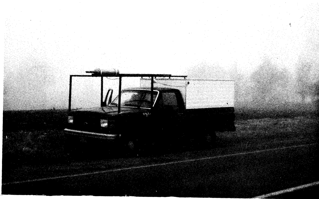
Fig. 2. Photograph of the ground-based vehicle at the field site, with FSSP mounted on its front.
