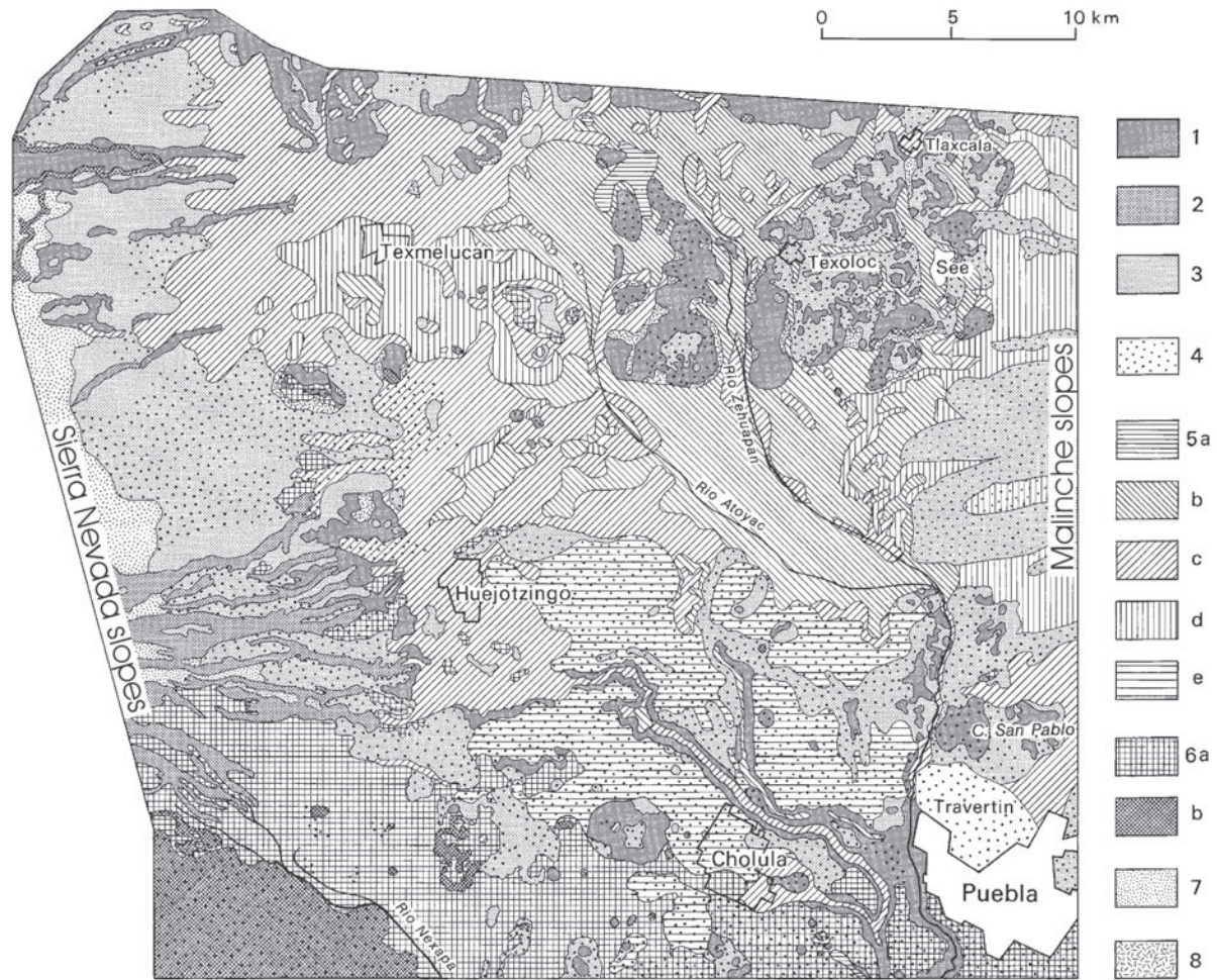
Figure 2. Erosion and accumulation in the basin of Puebla–Tlaxcala. Interpretation of a color soil map published by Aepli and Schönhalz (1975). 1: Erosion of top soil down to extremely cemented tepetate horizons or bed rock; 2: Development of deep barrancas (gullies); 3: Linear and sheet erosion, yet thin soil profiles are present; 4: eolian sandy cover sediments; 5: fluvial accumulation (alluvial soils), a) clay, b) silt, (c) sand, d) gravel, e) lake sediments; 6: volcanic sedimentation, a) sand, lapilli, breccia, b) lava flows; 7: volcanic ash soils (Andosols) on slopes above 3,000 m a.s.l. with different erosion features caused by human activities; 8: slope colluvium.
